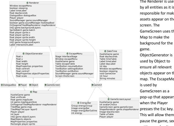
The Renderer is used by all entities as it is responsible for making assets appear on the screen. The GameScreen uses the Map to make the background for the ObjectGenerator is used by Object to ensure all relevant objects appear on the map. The EscapeMenu is used by GameScreen as a pop-up that appears This will allow them to pause the game, see settings and quit.
